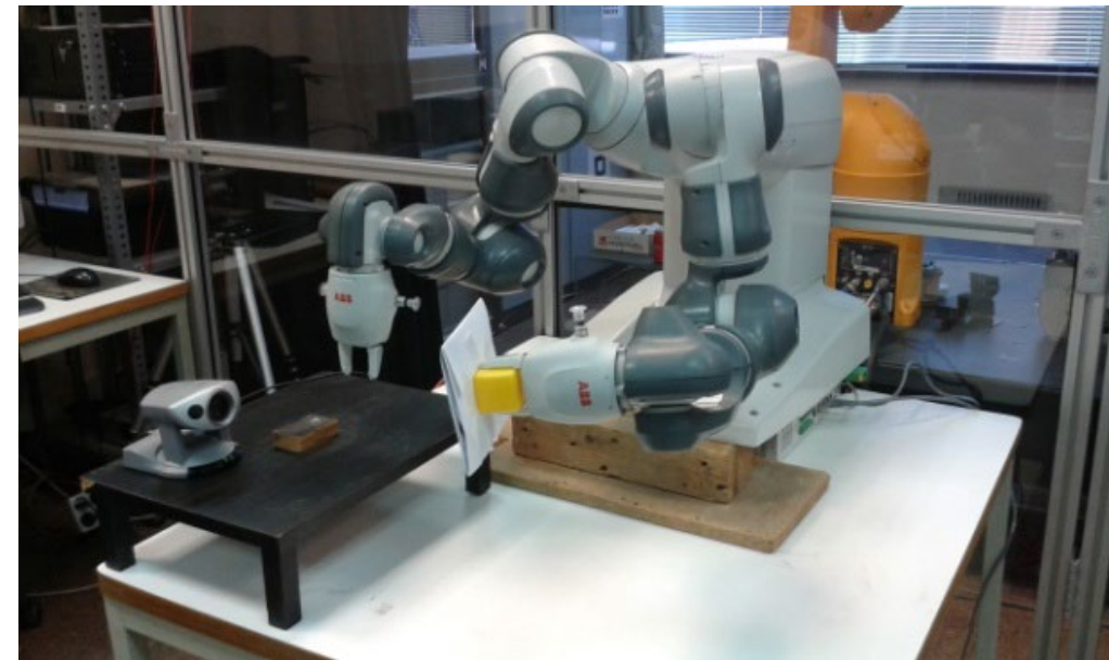
Implementation of a visual servo control in a bi-manual collaborative robot.
